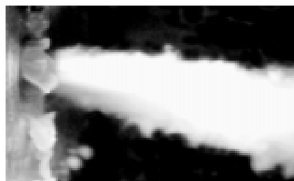
Figure 9. Jet through porcine valve: image obtained with light-sheet illumination, Re=8250 .
