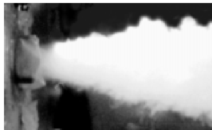
Figure 8. Jet through bovine pericardium valve: image obtained with light-sheet illumination, Re=8250 .
