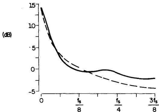
Fig. 2 - Amplitude response of IIR approximation (solid line) to theoretical  $1/\sqrt{f}$  response (broken line).
