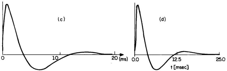
Fig. 3 - Amplitude response of Koch's (1984) cable transfer function (a) and of the third order linear approximation (b). Impulse response of the approximation (c) and the original impulse response (d) of Koch (1984).
