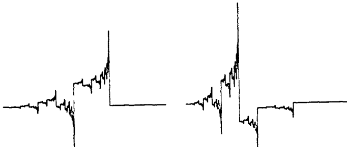
Fig. 6. \phi(x) and \psi(x) for the wavelet with 4 samples and \nu=1.5 .
