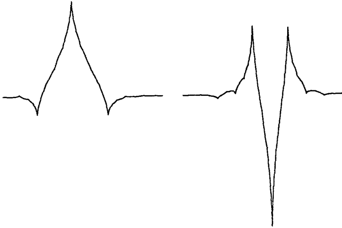
Fig. 7. \phi(x) and \psi(x) for the wavelet of with 6 samples and \alpha=1.15 , \beta=0.4 .
