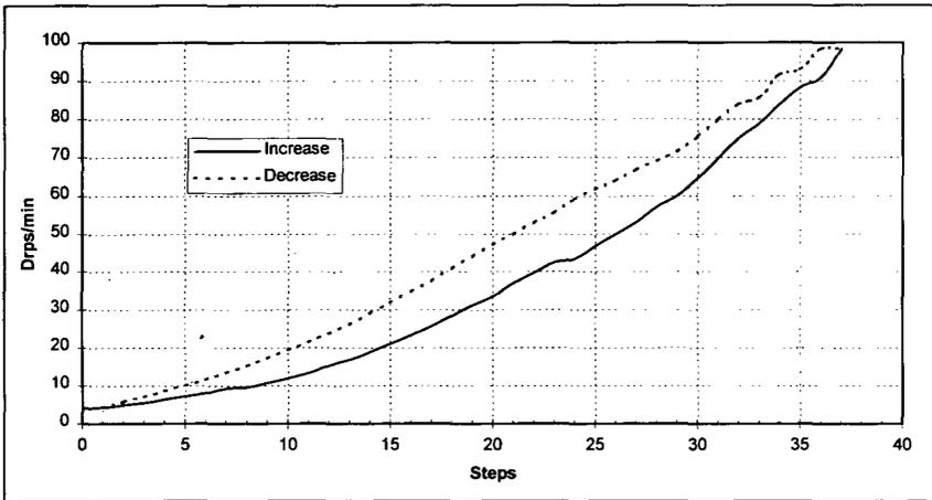
Figure 2. Graph of the hysteresis from 0 to 98 drop/min flow rate (dotted line = compression of the plastic tube ; solid line = opening of the pincer jaws).
