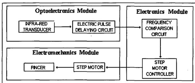
Figure 2 - Block diagram of the programmable controller.
