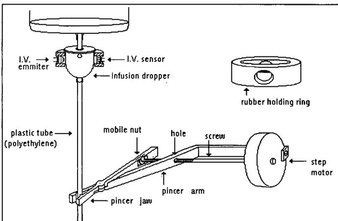
Figure 1- View of the main mechanical components of the controller.
