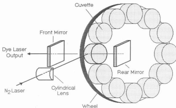
Figure 1. Nitrogen pumping dye laser configuration.
